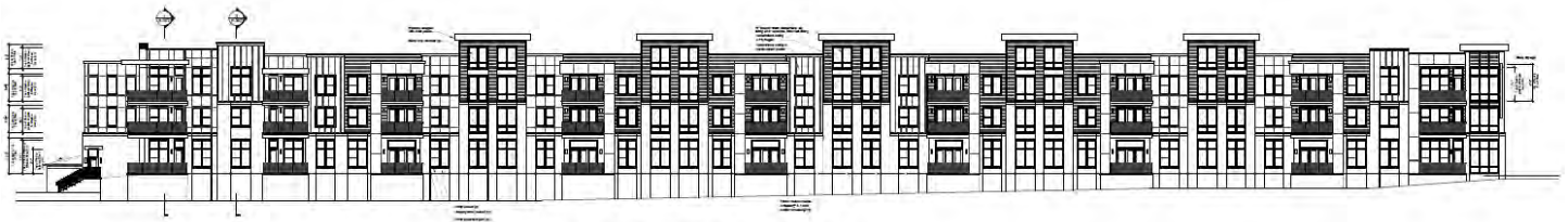
1 Building 1 Front Elevation Scale: 1/8" = 1'-0" Type: 9A Construction
