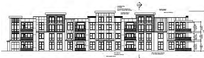
1 Building 4 Front Elevation Scale: 1/8" = 1'-0"
